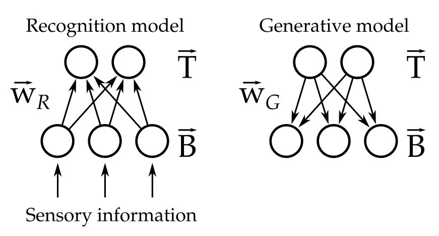
The simplest Helmholtz machine is composed of binary stochastic units arranged in a bottom layer  $\vec{B}$  and a top layer  $\vec{T}$ . These two layers are interconnected with two separate sets of connections (with weights  $\vec{w}_G$  and  $\vec{w}_R$ ) creating two independently functioning networks. The bottom-up connections implement the recognition model used for inference. The top-down connections implement the generative model.
